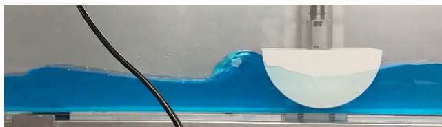
Figure 33: Wave breaking at the wave generator. The downward-moving plunger displaces too much water in a short period, forcing some water to break the surface. This wave breaking leads to extra fluctuations and must be avoided.
