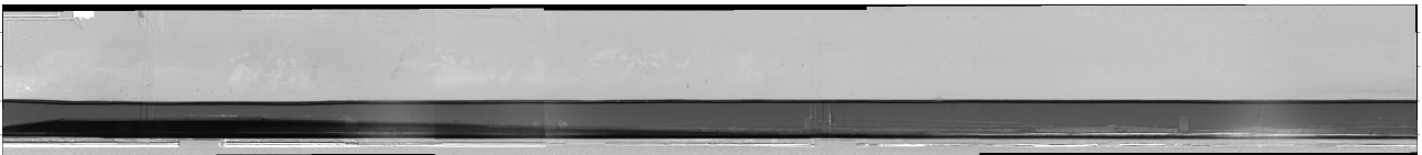
Figure 62: Composite image consisting of 3 stitches camera frames of the setup containing the linear slope. The darkest shade is the slope, the darker shade is the water and the lighter shade is the air.
