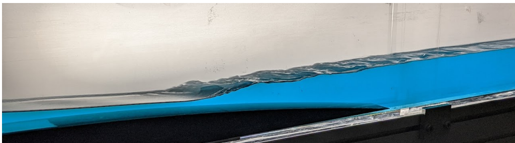
Figure 64: Supercritical ( \text{Fr} > 1 ) to subcritical ( \text{Fr} < 1 ) flow transition generating a hydraulic jump and resulting in turbulence in the obstacle wake.
